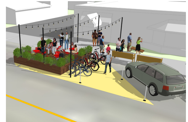
A rendering of the Pilot Project highlights: planters, bike parking, a parklet, diagonal parking and benches.
