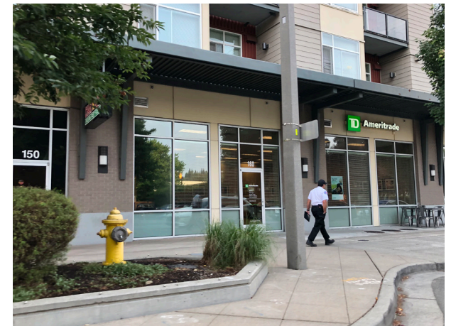
In this example, the curb extension provides additional space for landscaping elements and sidewalk space and could also be used for stormwater collection.
